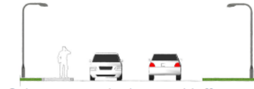
Curb and gutter in a local street with buffered sidewalk on one side
