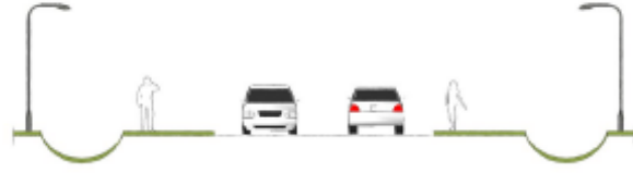
Open ditch next to property line with no sidewalks
