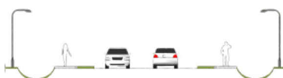
Open ditch next to property line with sidewalk on both sides
