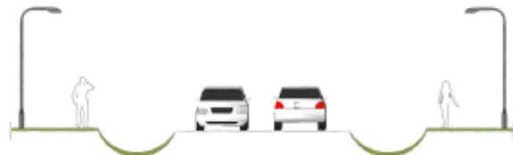
Open ditch between narrow roadway or property line
