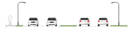
Curb and gutter in a major thoroughfare with buffered sidewalk on one side
