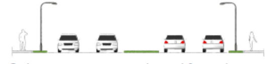
Curb and gutter in a major thoroughfare with buffered sidewalks on both sides
