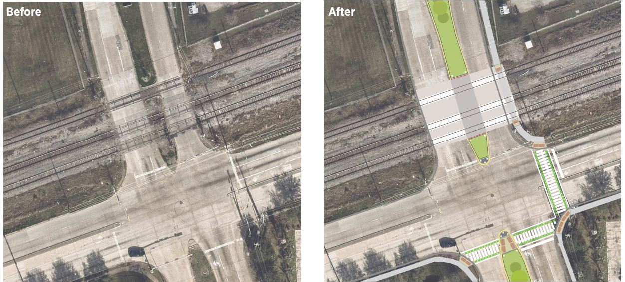
Figure 20, Holmes Road/Fannin Street Intersection Improvements
