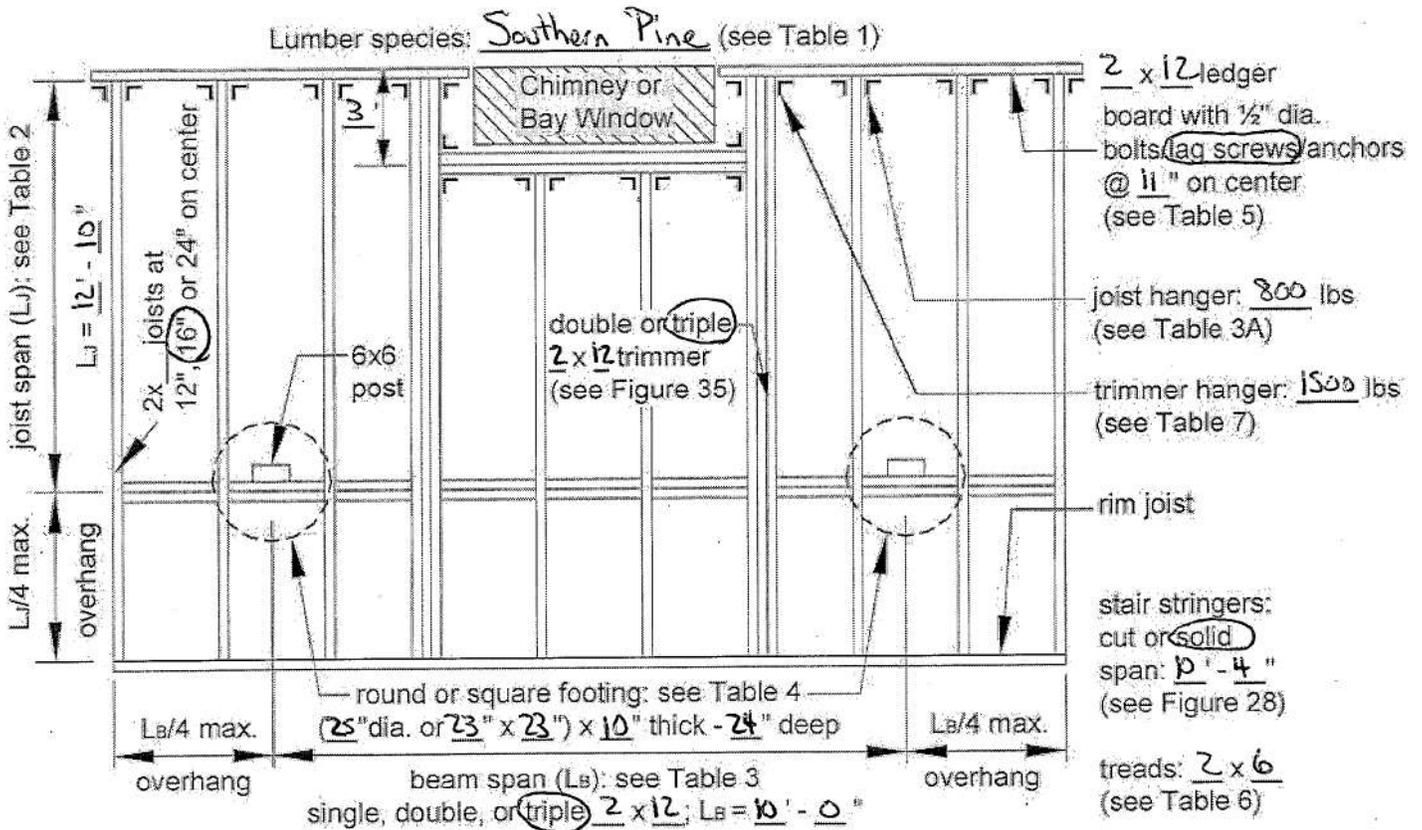
**Figure C5. Example of Typical Deck Framing Plan**
