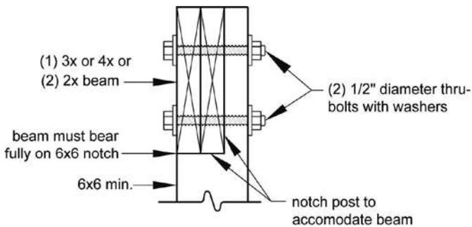
**Figure 9. Prohibited Post-to-Beam Attachment Condition**
