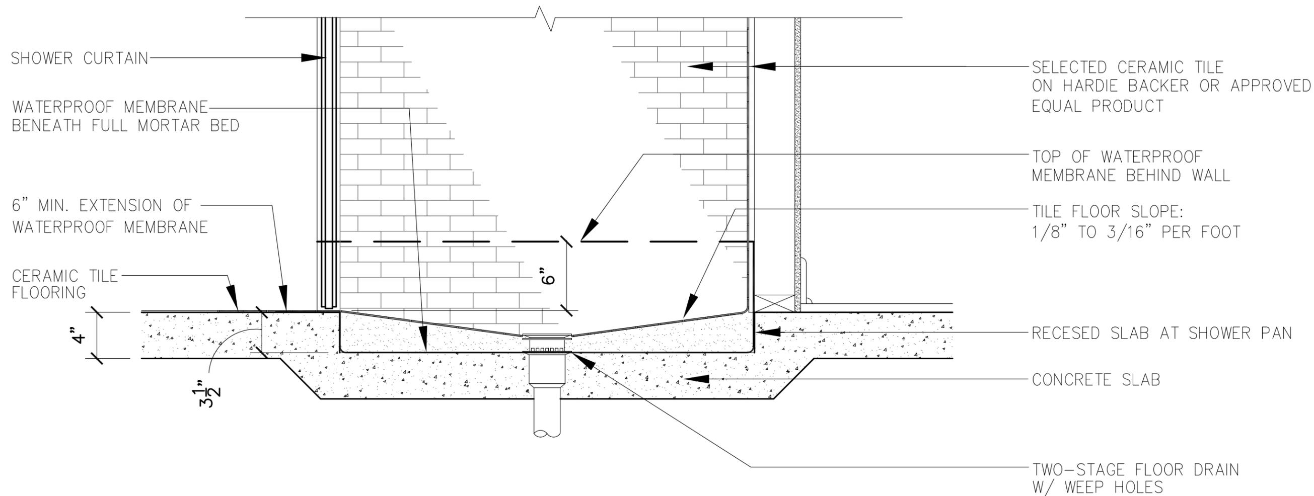
SHOWER DETAIL AT RECESSED CONCRETE SLAB ON GRADE FOUNDATION
