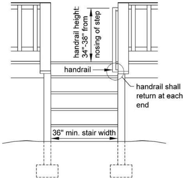
**Figure 34. Stair Footing Detail**
