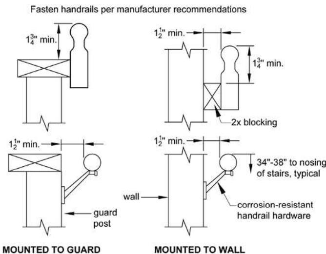
**Figure 32B. Handrail Grip Size**
