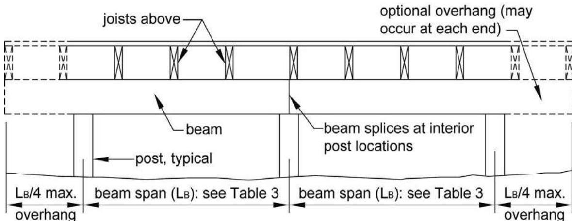
Figure 4. Beam Assembly Details
