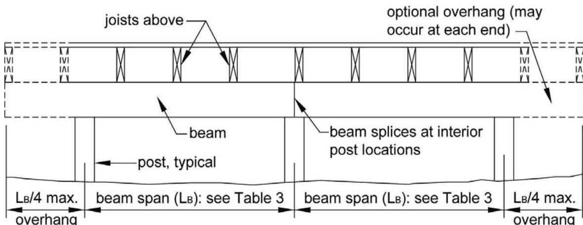
Figure 4. Beam Assembly Details
