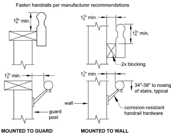
**Figure 32B. Handrail Grip Size**
