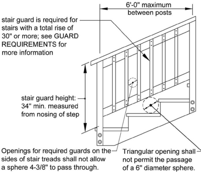
**Figure 31. Stair Stringer Attachment Detail**
