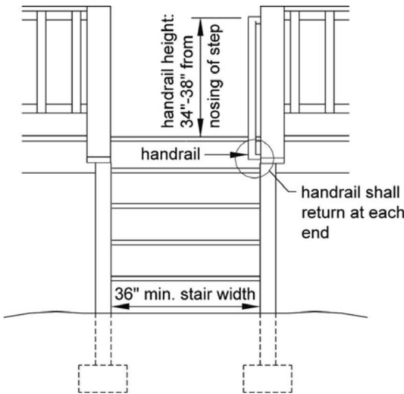
**Figure 34. Stair Footing Detail**
