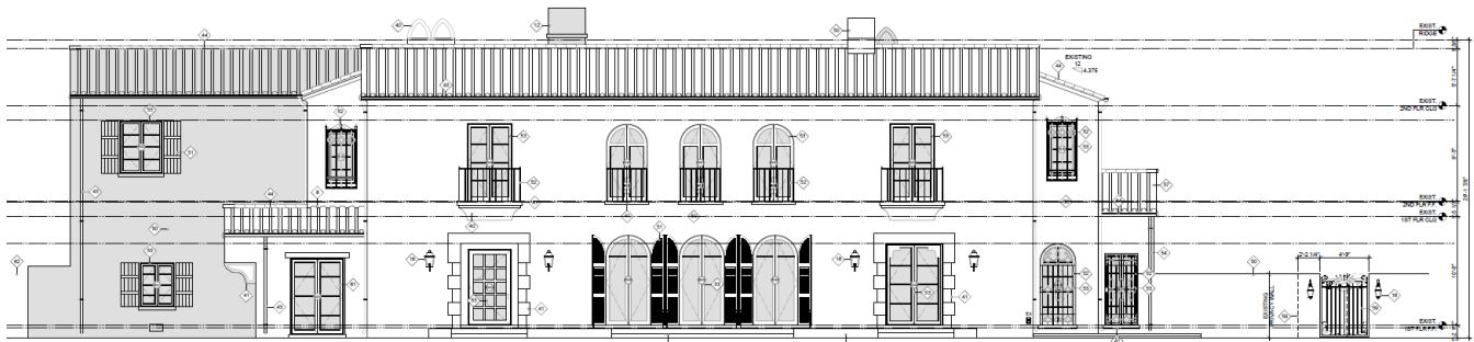
01 PROPOSED SOUTH EXTERIOR ELEVATION SCALE: 1/8"=1'-0"
