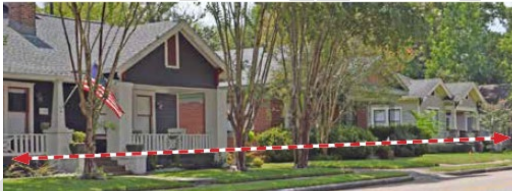
Maintain the historic height of the finished floor above natural grade, if possible. This is a key feature of the building and the context.
