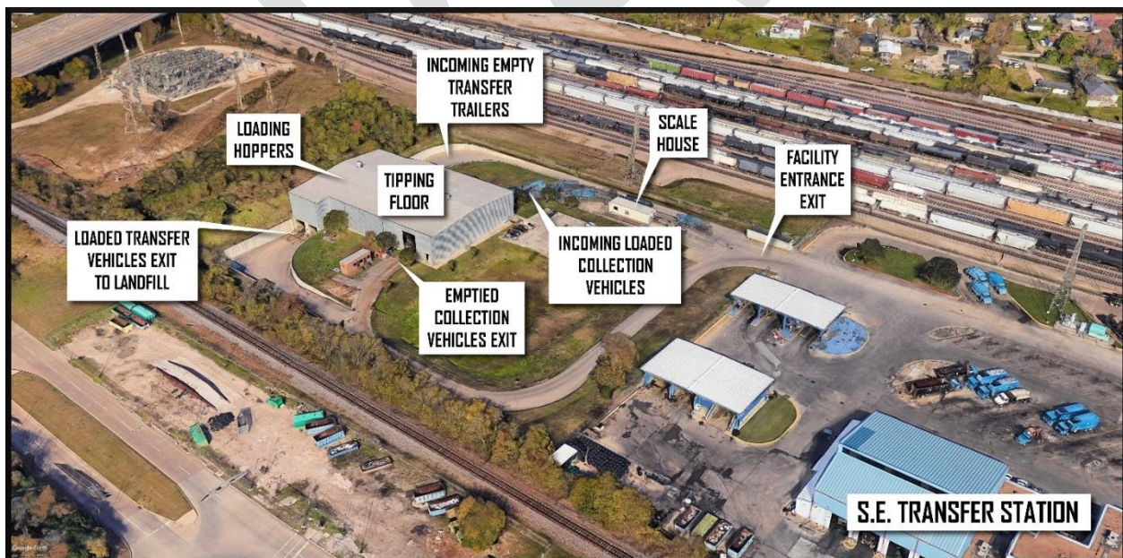
Figure 6-1 SE Transfer Station Layout
